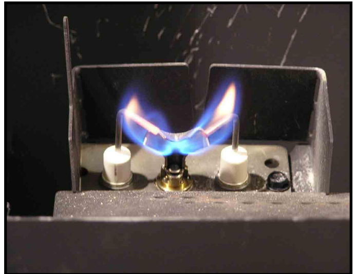
Figure 3.1 - IPI Pilot Flame Patterns
