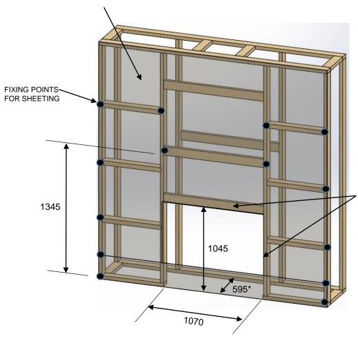
NO FIXING OF SHEETING TO THE HEADER OR NEAREST STUD TO THE FIRE APPLIANCE. USE SELLEY'S 401 SILICON TO ADHERE TO THE NEXT AVAILABLE STUD OR HEADER.
