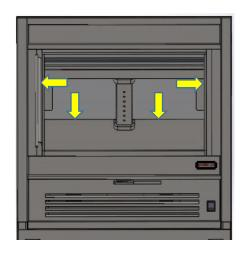
4. REPEAT THE PROCESS FOR THE OTHER SIDE. PUSH BOTH BAFFLE PLATES UNTIL IT IS AGAINST THE SIDE AND REAR WALLS.
