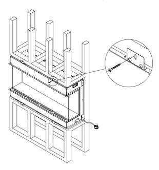
5.7a3 Cover the framework by panels or plaster board, it can be used directly against the sides and front of the appliance.
