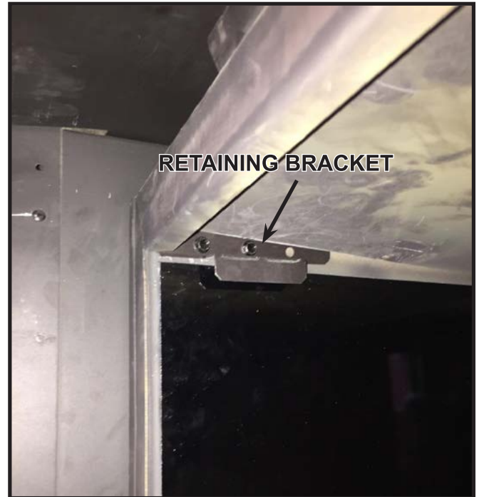
Figure 11.6. Retaining Bracket Installation - Single-sided Models
