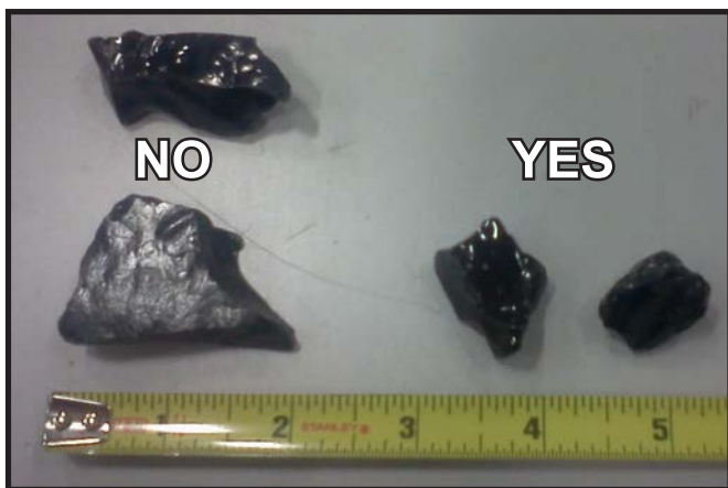
Figure 11.8 Selecting Flat Media for Pilot Cover.
