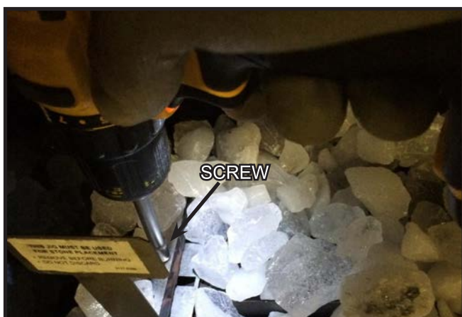
Figure 11.12 Remove Media Placement Jig
