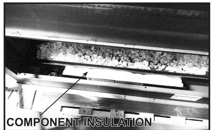
Figure 11.3 Component Insulation Location
