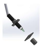
REMOVE ALL WASHERS AND NUT FROM THE WIRING. THEN ATTACH THE BULB TO THE LIGHT FITTING.
