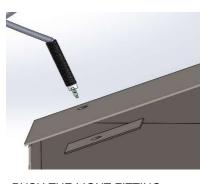
PUSH THE LIGHT FITTING THROUGH THE HOLE ON THE OUTER BOX AND INTO THE GAP BETWEEN THE PLATE AND OUTER BOX.
