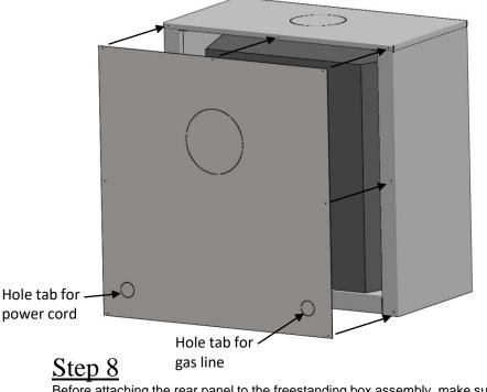
Before attaching the rear panel to the freestanding box assembly, make sure the power cord and gas line hose exits through the rear panel holes. Push out the hole tabs as required. The gas line connector can be accessed through the front of the unit. Screw the rear panel on and the assembly is complete.
