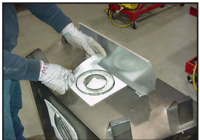
Figure 6.5 Remove the seal cap.
