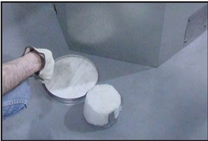
Figure 6.12 Discard the seal cap, remove and discard the insulation basket.
