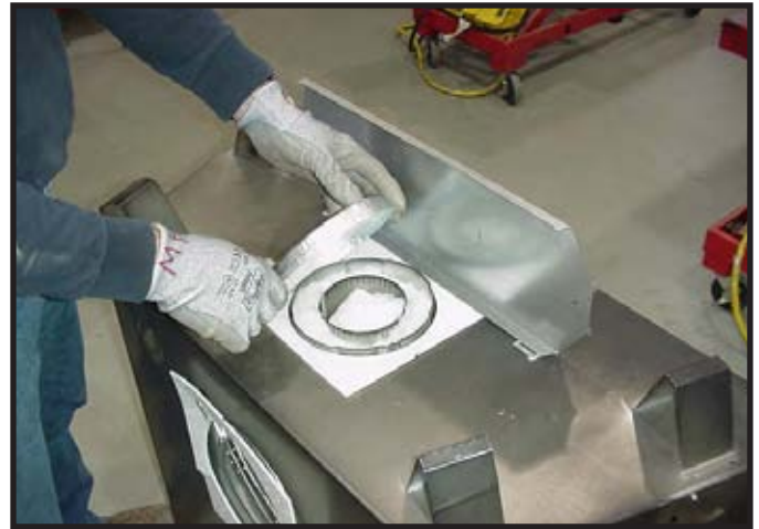
Figure 6.4 Remove the seal cap.
