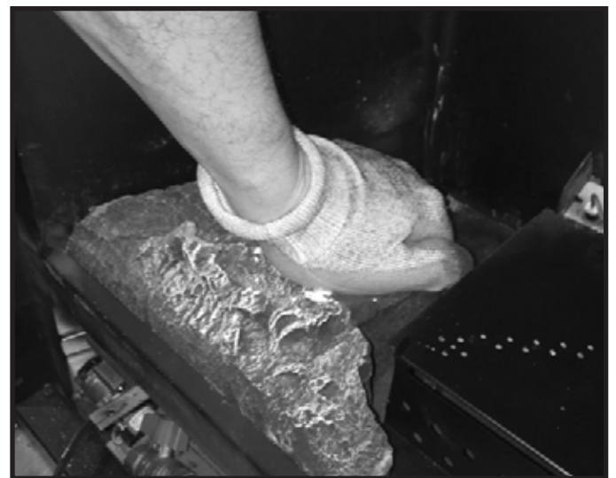
Figure 11.2 Press Left Hearth Firmly Into Place
