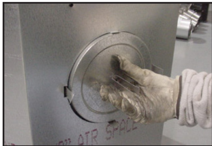
Figure 6.10 (Generic Appliance Shown) Fold the center parts of the retaining band out and use to remove the seal cap.
